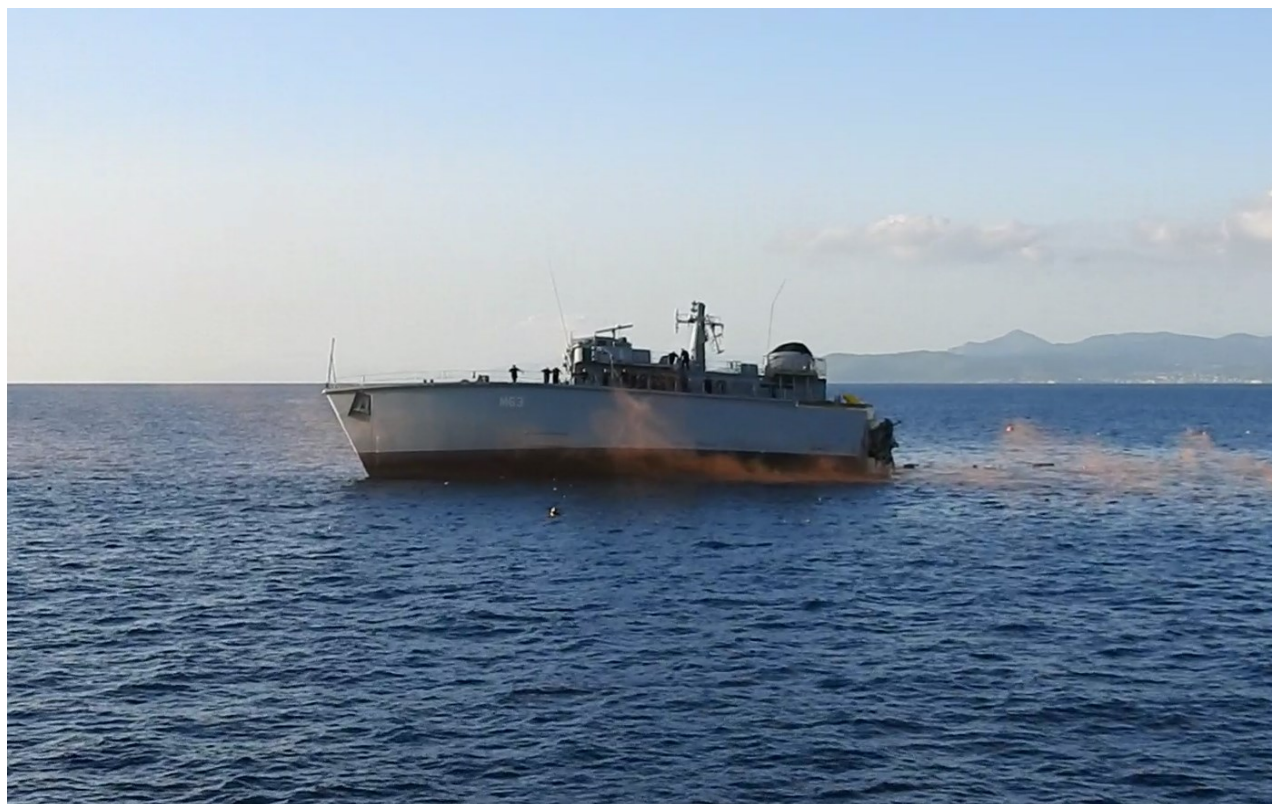
Figure 17. The fore part of HS KALLISTO listed to her starboard side.
